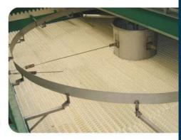
The unique design of crisscross structure can bear more than 500 kg of dead load, greatly extending the service life and save expenditures. The tilt angle of HPVR series is 60 degrees, and H / h is 6, which is two times more than that of the single-row structure. Therefore, floc particles in the fluid will not be attached to the pipe surface during precipitation, rectification and secondary coagulation, and functions of the slanting pipes are accordingly improved.
